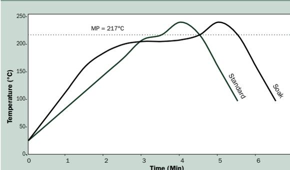
The stated profile recommendations apply to most Pb-Free alloys in the Sn/Ag/Cu (SAC) alloy system, including SAC 305 (96.5Sn/3.0Ag/0.5Cu). This can be used as a general guideline in establishing a reflow profile when using **Indium8.9** Solder Paste. Deviations from these recommendations are acceptable, and may be necessary, based on specific process requirements, including board size, thickness & density.
